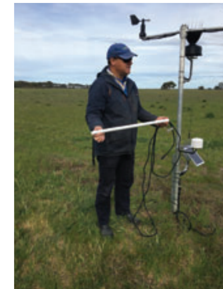
Automated soil moisture probes, salinity and depth sensors with data transfer units were installed as part of the nbn™ Sustainable Agriculture Landcare project to measure the depth of the water table, soil moisture levels, soil salinity levels and environmental conditions across the project's three sites.
